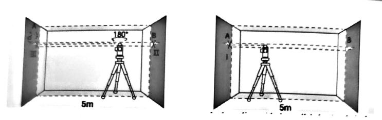
Align the laser line with the wall A that is relatively close, level the measuring instrument, rotate the measuring instrument 180 degrees, and level the instrument, find out the X-Crossing point of the laser line on the wall A, mark the center of the X-Crossing point on the wall B, and mark point I on the center of the X-Crossing point.
